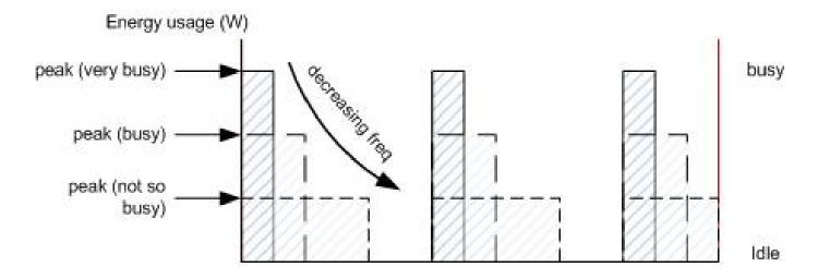
A P-state is an operational state; the core can be doing useful work in any P-state. P0 has highest operating frequency and voltage.
