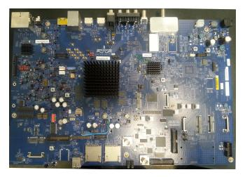
Figure 5: Broadcom BCM97445VMS Board with an BCM53125 Switch at the top-left
