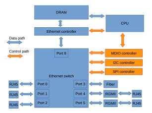
Figure 1: The Basic DSA setup
