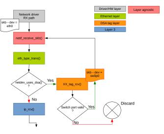
Figure 11: Processing the Switch Tag
