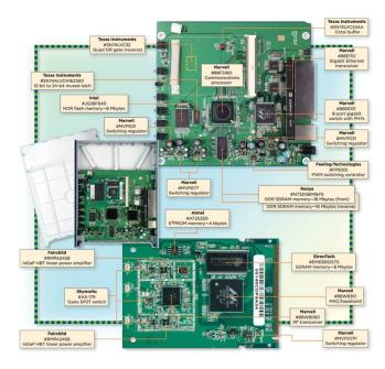
Figure 4: Annotated WRN854T WiFi Access Point, image from OpenWrt
